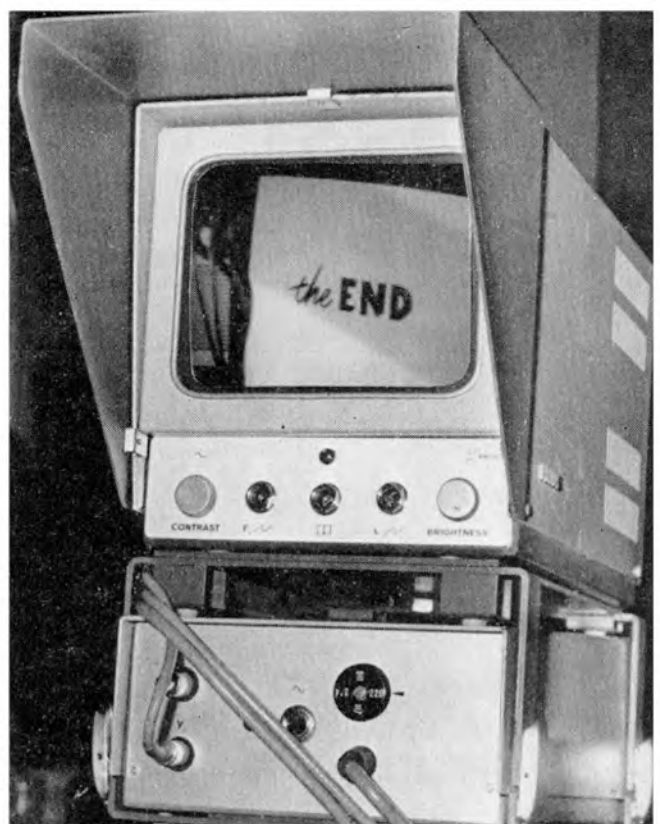
View of the electronic monitor mounted on the VTR camera
