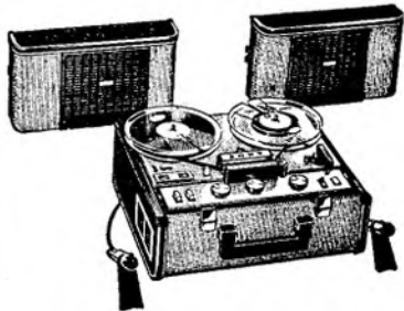
TC-200. Complete 4-track stereophonic and monophonic tape recording system. 2 full range balanced speaker systems. Sound-on-Sound. Variable tone control. 2 VU meters. Tape index counter. Instant stop, individual track selection. Recording monitor. Transistorised pre-amplifier. Individual level controls on each channel. Complete with 2 dynamic microphones 72 Gns.
