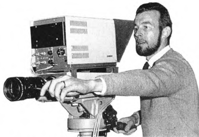
Fred Chandler operates the Peto-Scott Video-Compact Camera, seen with the electronic monitor mounted above
